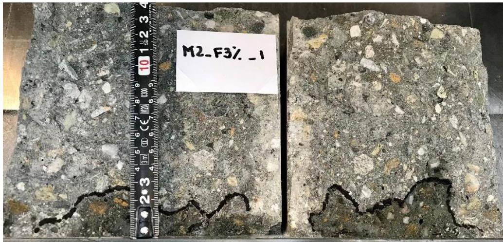
Figure 21. Marked front of water penetration in a concrete specimen with 3% of CaCO 3 addition.
