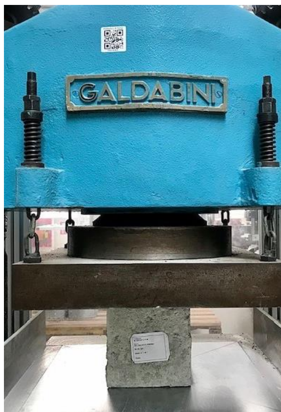
Figure 19. Compression test on the hardened concrete
