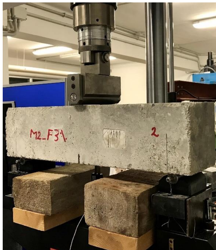
Figure 22. Three-point bending test on the hardened concrete
