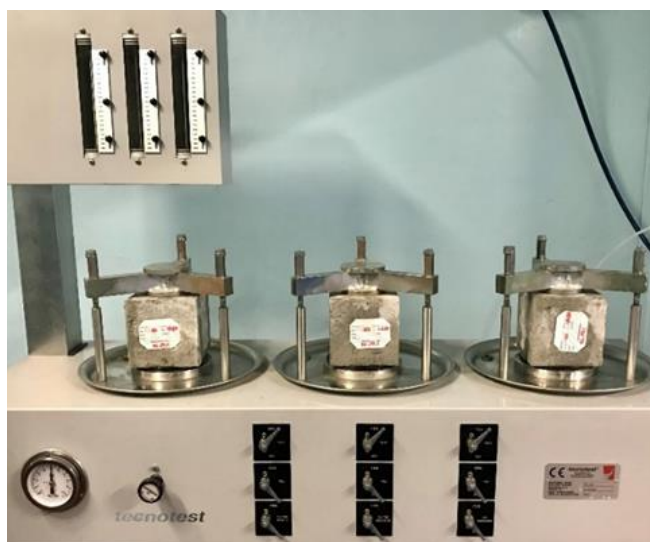
Figure 20. Test of the depth of penetration of water under pressure on the hardened concrete
