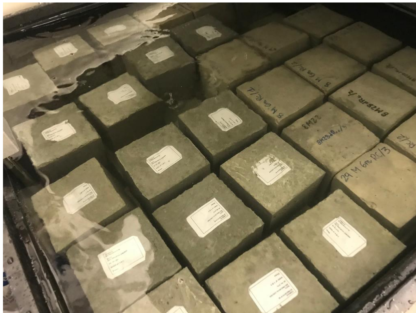
Figure 18. Concrete specimens curing
