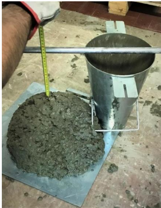
Figure 17. Slump test on the fresh concrete
